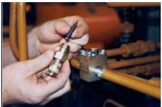
•Screw out the sampling valve and remove the spring plug, needle and pressure disk.
