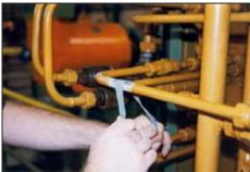
•Check to see that the line is pressureless and the machine is shutoff and locked out.
