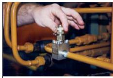
•The sampling valve is screwed back in and the system is ready for use.
